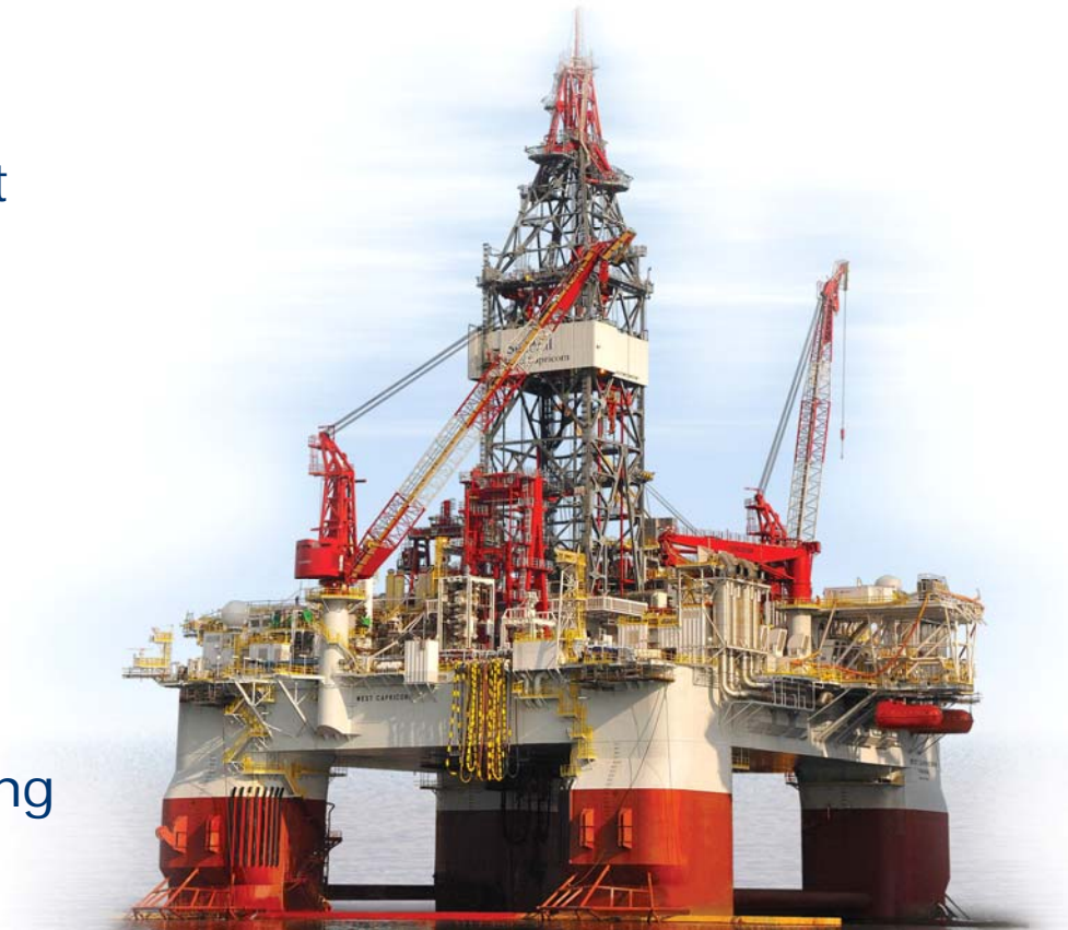
6 th gen. semi-submersible rig West Capricorn
